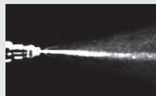
Injector spray pattern before P.i. treatment.
