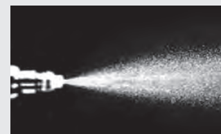
Injector spray pattern after P.i. treatment.
