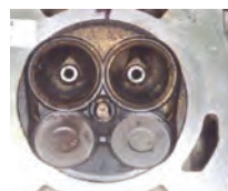
Combustion chamber before P.i. treatment.
