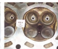
Combustion chamber after P.i. treatment.
