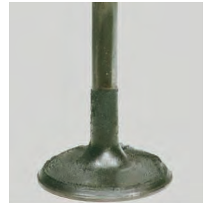
Picture E - Intake valve after P.i. treatment
