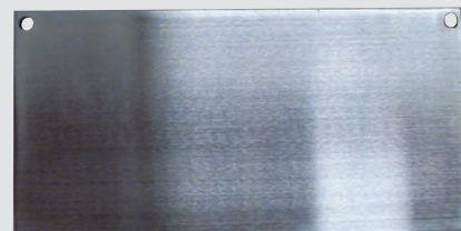
After 192 hours in a humidity cabinet, the metal coupon treated with Z-ROD Synthetic Motor Oil showed no signs of rust or corrosion.
